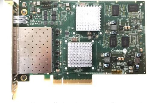
The host machine should support PCIe bifurcation to enable all the 4 Ports of T6425-CR. Otherwise, only 2 ports will be enabled. It runs all the host software of its predecessor, T5, as-is, thus enabling leveraging of all the prior software investment. It offers all the features of T5, and in addition adds support for integrated offload of IPsec, TLS/SSL, DTLS and SMB 3.X crypto.
